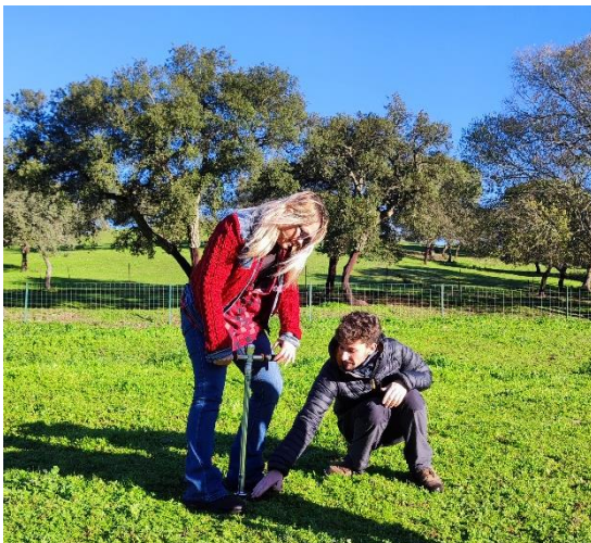
Figure 3: Bulk density; sampling with Kopecky rings
