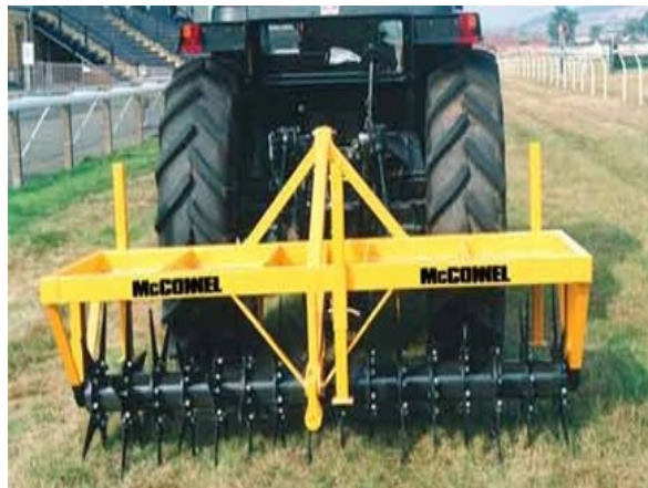
Fig.1: Example of an aerator or spiker/ slitter
