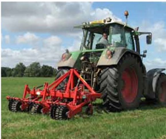
Fig.2: Example of a sward lifter
