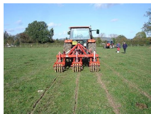
Fig. 4: Ground surface and sward after sward lifting
